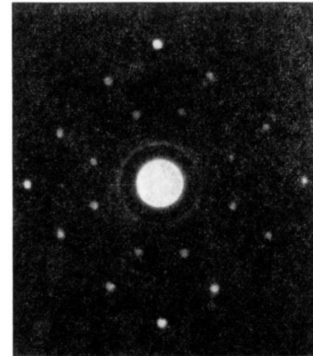
FIG. 1. Laue photograph showing neutron diffraction by NaCl.
